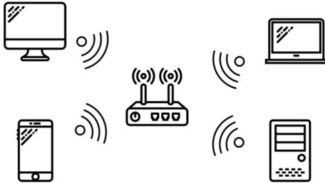
Figure 1: Computing devices contain wireless adapters which communicate with an access point (shown at center).
