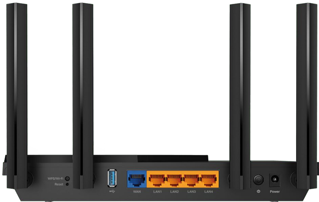
Figure 2: Gateways feature built-in Ethernet switches, as you see here at the center of this TP-Link Archer AX55.
